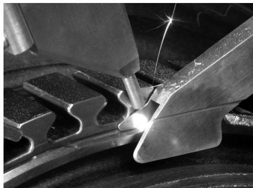
Left: High value components suitable for the repair with Laser Metal Deposition (Photo: Rolls-Royce Deutschland Ltd. & Co. KG).
