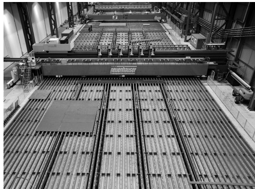
Left: View on the new one-side-welding station, on which panels by a size up to 30 x 25m are constructed (Photo: MEYER WERFT Laserzentrum GmbH, Papenburg). Right: Automated systems of the new panel line of MEYER WERFT at one view. (Photo: MEYER WERFT Laserzentrum GmbH, Papenburg)
